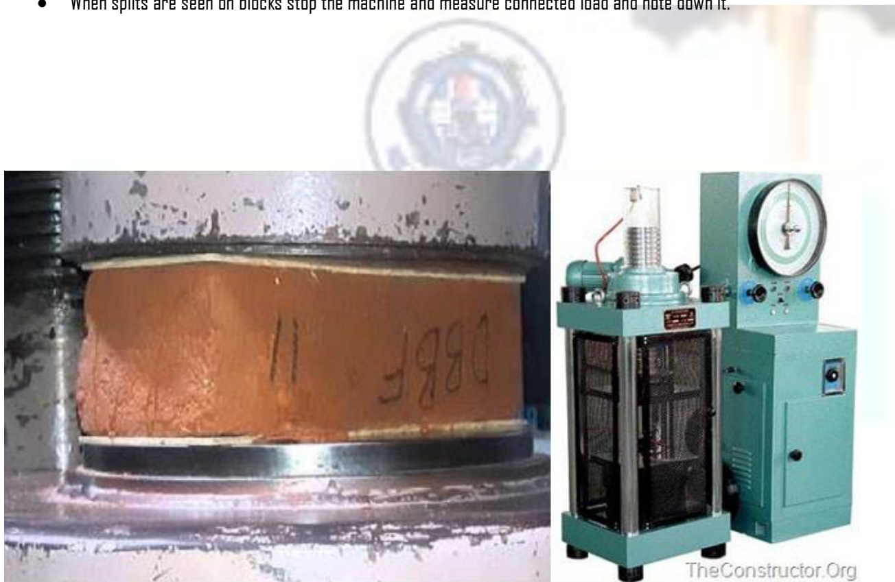
Figure 4: Compressive strength test
